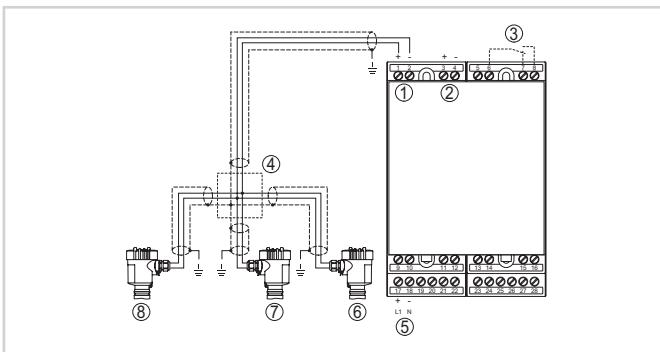
Connection example VEGASCAN 693 with two-wire sensors
