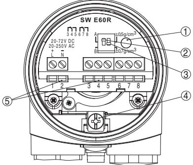
Electronics and connection compartment, single chamber housing
