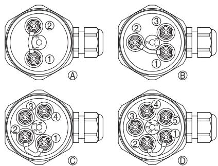
Connection compartment of the probe - 220 kΩ resistance between terminals 1 and 2
