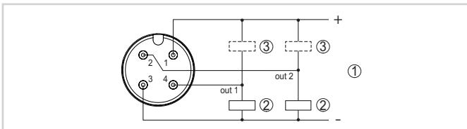
Wiring plan M12 x 1 plug - Transistor output, three-wire
