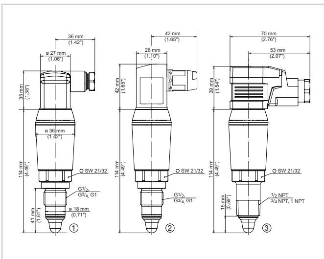
VEGAPOINT 21, standard version - thread with valve plugs acc. to ISO 4400
