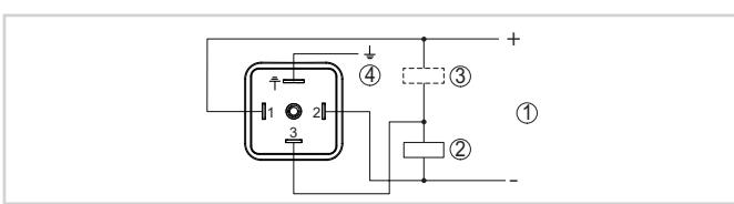
Wiring plan ISO 4400 plug - Transistor output, three-wire
