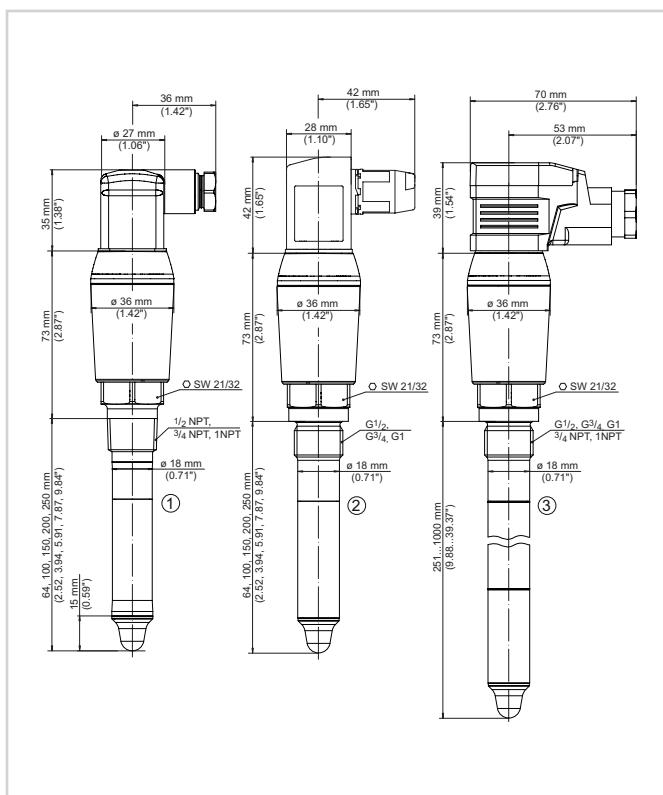
VEGAPOINT 23, standard version - thread, with valve plugs acc. to ISO 4400
