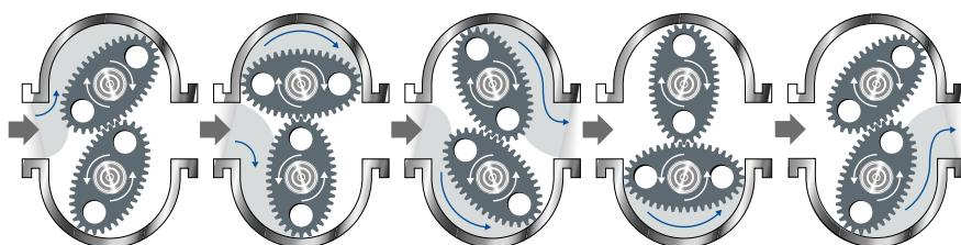
A conversion coefficient, specific to each meter size, enables the conversion of this frequency into a flow rate. The standard K-factor depending on the meter size is available in the flowmeter's operating instructions, see **Type 8071** ▶. To improve the measurement deviation, a device-specific K-factor is given on the device label.
