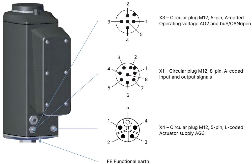
The following circular plug-in connectors are used depending on the device variant:
