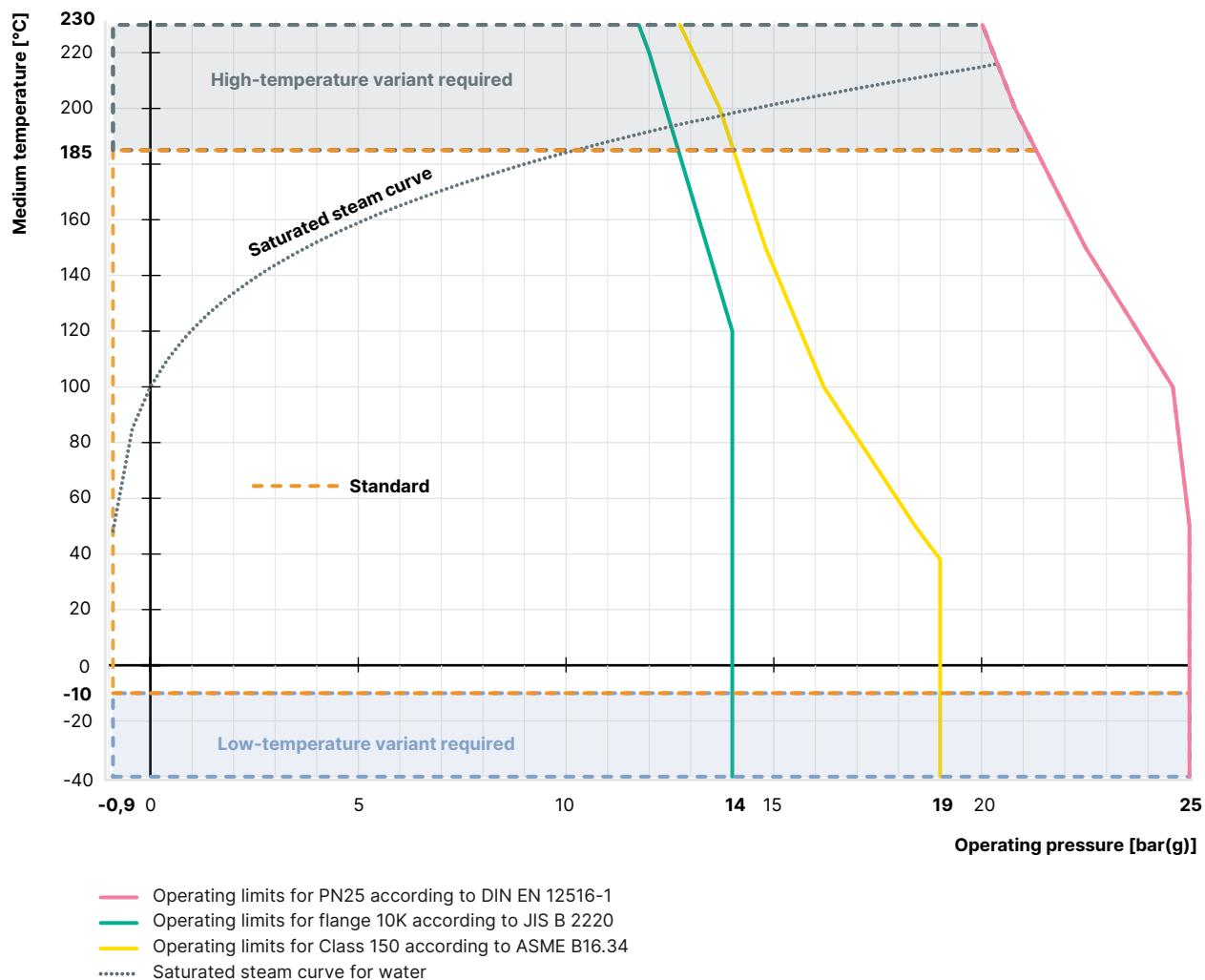
**Operating limits for ambient and medium temperature**
